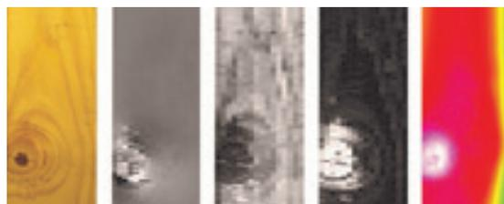
(left to right) colour, tracheid scatter, tracheid angle, knot detection, profile: (left to right) colour, tracheid scatter, tracheid angle, knot detection, profile
